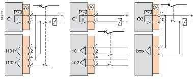
Connection for shunt trip coil monitorina.
