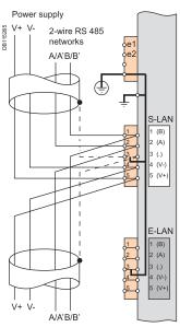
If ACE969TP and ACE969TP-2 are used together, the external power supply is required.
