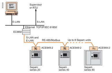
Note: Rc = line-impedance matching resistor.
