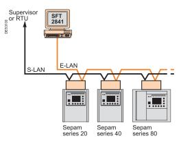
Sepam connection to two communication networks (S-LAN and E-LAN).
