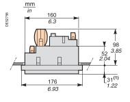
Sepam with advanced UMI and MES114, flush-mounted in front panel.
