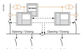
Automatic transfer with synchro-check controlled by Sepam series 80.
