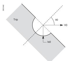
Tripping characteristic of ANSI 67N/67NC type 2 protection (characteristic angle g0 ¼ 0°).
