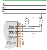
This variant does not allow the calculation of residual voltage.
