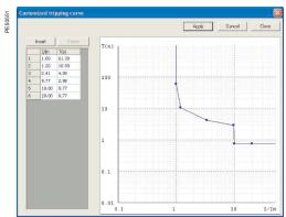
Customized tripping curve set using SFT2841 software.
