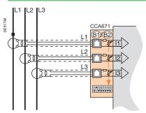
Connection of 3 Low Power Current Transducer (LPCT) type sensors to the CCA671 connector. It is necessary to connect 3 sensors; if only one or two sensors are connected, Sepam goes into fail-safe position.
