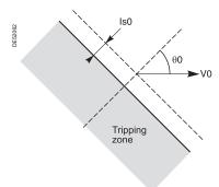
Tripping characteristic of ANSI 67N/67NC type 1 protection (characteristic angle q0 0°).
