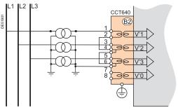
Measurement of the 3 phase-to-neutral voltages allows the calculation of residual voltage,  $V'0\Sigma$ .
