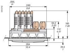
Top view of Sepam with MES120, flush-mounted in front panel with spring clips. Front panel: 1.5 mm (0.05 ln) to 6 mm (0.23 ln) thick.
