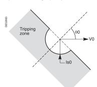
Tripping characteristic of ANSI 67N/67NC type 2 protection (characteristic angle q0 0°).
