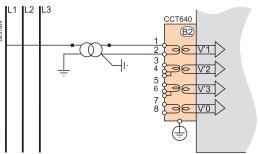
This variant does not allow the calculation of residual voltage.
