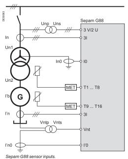
Sepam series 80 has analog inputs that are connected to the measurement sensors required for applications:
