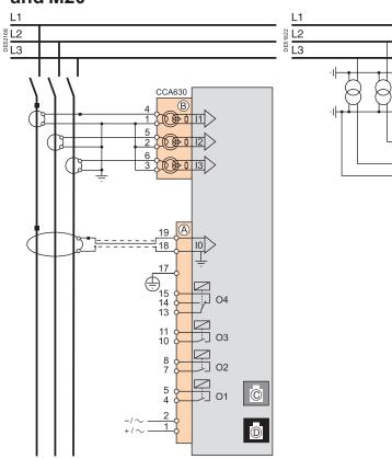
(1) This type of connection allows the calculation of residual voltage.
