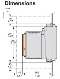
Side view of Sepam with MES120, flush-mounted in front panel with spring clips. Front panel:  $1.5\,\mathrm{mm}$  ( $0.05\,\mathrm{ln}$ ) to  $6\,\mathrm{mm}$  ( $0.23\,\mathrm{ln}$ ) thick.
