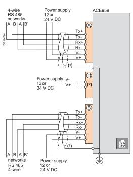
(1) Distributed power supply with separate wiring or included in the shielded cable (3 pairs).
