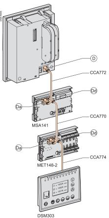
Example of inter-module linking on Sepam series 20.
